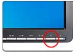
Hotkey of Input Select for switching among HDMI / Component / DVI / VGA signals
