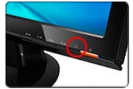
Hotkey of Input Select for switching among HDMI/ DVI/ VGA signals
